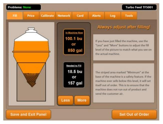
Three step calibration allows you to quickly calibrate your machine to the weight differences of wet or dry corn. If you prefer to adjust these values manually you can do that too.
