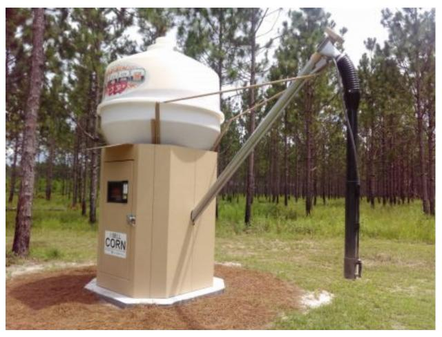
The chute handle allows customers to stop and start the flow of corn to fill multiple containers, the same can be done from the touch screen.
